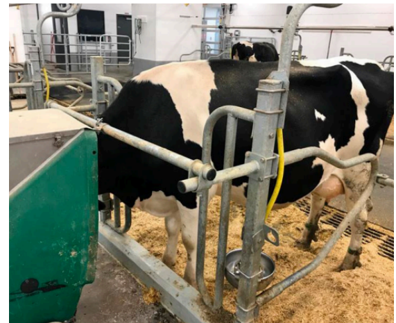
A dairy cow using a GreenFeed machine to have her emissions tracked while eating. PHOTO: KERRY HOULAHAN
